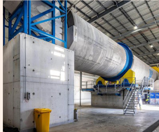
Australia's first drum pulper in Coolaroo, Victoria. Photo courtesy of VISY Industries.
